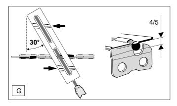
The file holder makes file guidance easier. It is marked for the correct 30° sharpening angle (keep the marks parallel with the chain when filing, see illustration) and limits the cut depth to the correct 4/5 of the file diameter. See "Accessories" for the order number.
